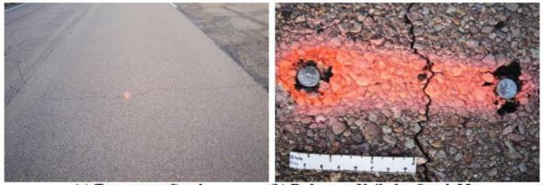
(a) Transverse Crack (b) Reference Nails for Crack Measurements Figure 8. Method for Measuring Crack Widths.
