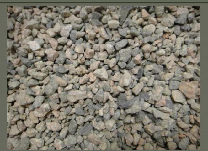
Mill Creek Aggregate (1/4-in chips) used by APAC at Dallas HMA Plants
